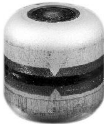
Figure 20 – Image of a Pu-238 fuel pellet in its protective iridium cladding. Image Credit: Dept. of Energy [54]
