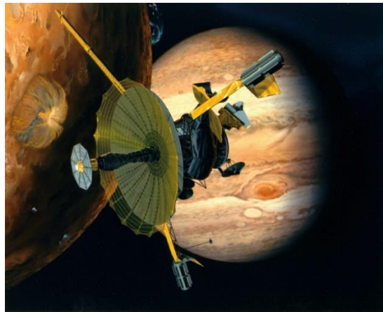
Figure 13 – Galileo Spacecraft Rendering with 2 GPHS-RTG's (in grey) on Booms [46]
